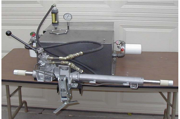
RPA 300 set up for testing rack and pinions
