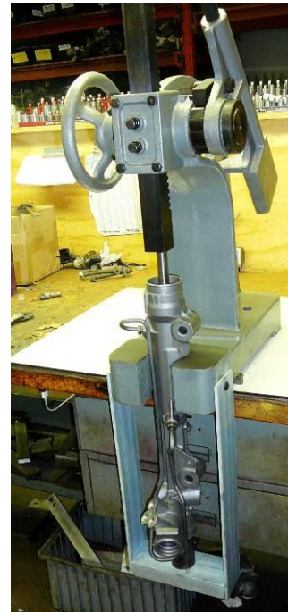
Pressing in Main Casting Seal in Assembly
