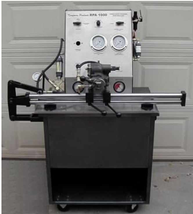
RPA 1000 set up for testing gearboxes
