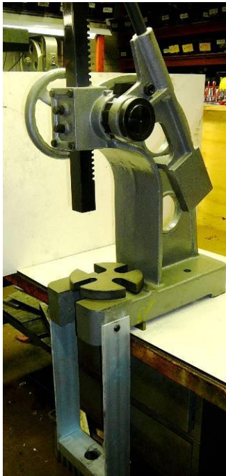
RAP 100 3 Ton Ratchet Arbor Press w/ Tooling
