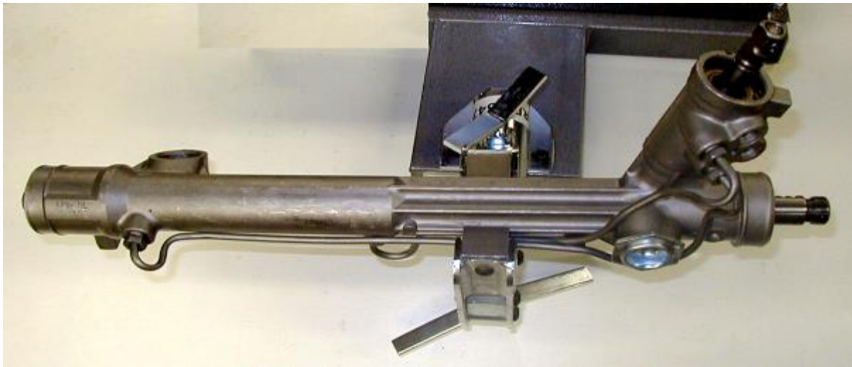
RPF 547 Rack Vise holding a rack
